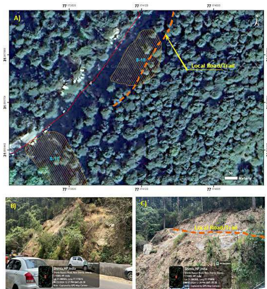
Image 4.24 - (A) Aerial view of rainfall triggered debris slide, (B and C) View of failure slope Note: There was exposed bedrock
