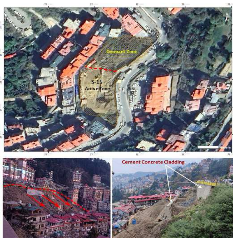
Image 4.31 - (A) Aerial view of the landslide area (note the active and dormant area), (B and C) View of landslide, settlements, and construction of retaining wall
