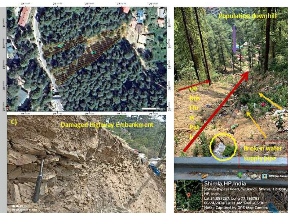
Image 4.2- Rain trigger debris flow partly caused by man made reasons: (a) location, (b) debris flow path and location of the broken pipe, and (C) failure immediately to the road impacted NH5, forest, and population downhill.
