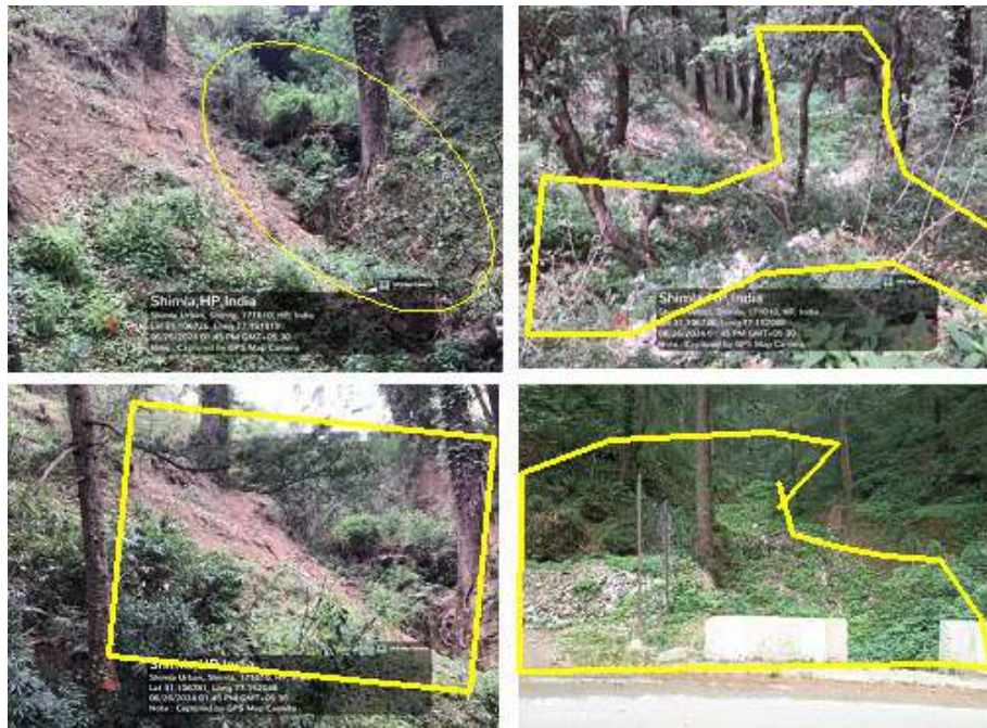
Image 4.42 - Incision of slope by streams followed by slope failure
