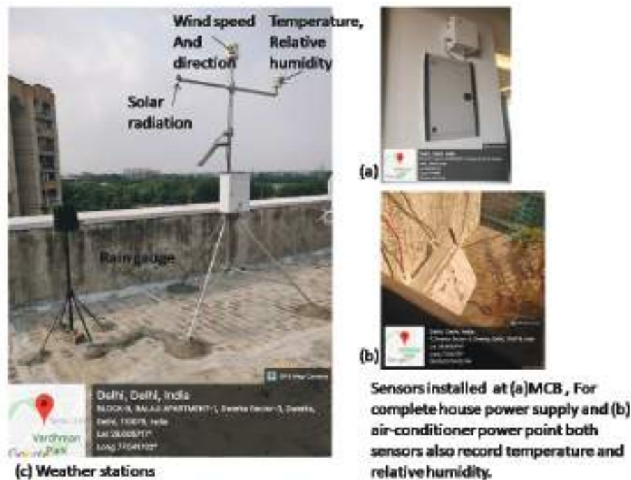
Figure 2. Sensors installed for power consumption and climate variables – indoor and outside environment
