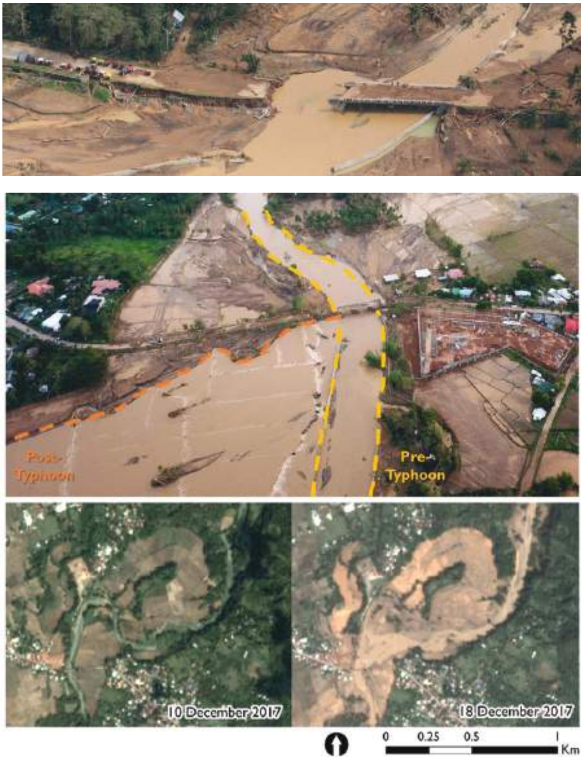
Figure 1. Damage associated with Typhoon Urduja (2017) on Biliran Island (Visayas) at Caraycaray Bridge
